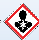
GHS 08 Respiratory sensitisation Germ cell mutagenicity Carcinogenicity Reproductive toxicity Specific Target Organ Aspiration hazard
